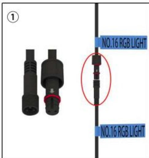
① Connect two led strip plugs with same labels. (Find out the arrows on the two cables and connect them, then tighten the caps.)
