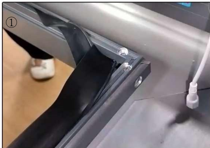
① Pull out the waterproof seals from the four corners of the drainage channel.
