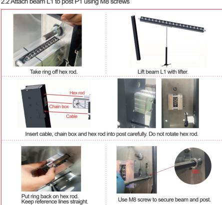
Use M8 screw to secure beam and post.
