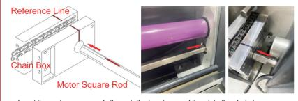
Insert the motor square rods through the bearings and then into the chain boxes. Keep the reference lines straight.
