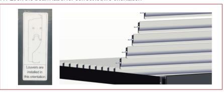
7.2 Place louvres onto gearboxes and secure them with M6 screws
